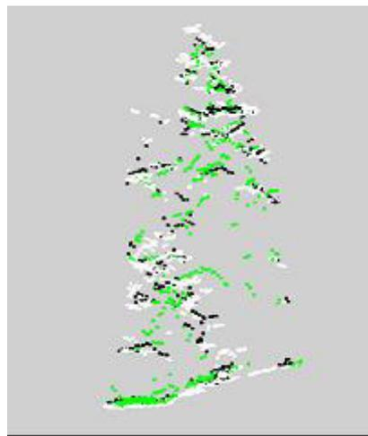
**Figure 4.** Growth of an individual tree measured using laser scanner and data acquisition performed in 1998 (green dots), 2000 (black dots), 2003 (white dots).
