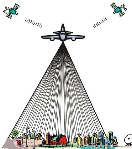
**Figure 1.** The principle of airborne laser scanning when applied to urban areas. The laser transmits pulses and determines the distance to the target based on the time spent. With the knowledge of the position and orientation of the laser beam when transmitted, the location of the reflected point on the target can be calculated.
