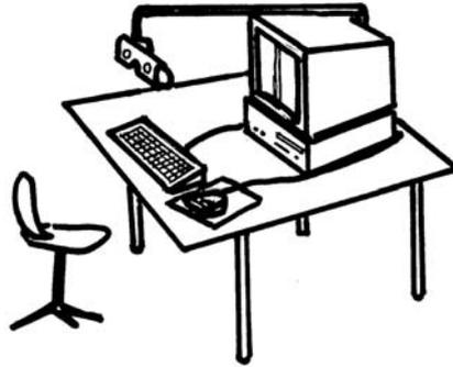
**Fig. 6.51 "Digital stereo-plotter scheme"**
