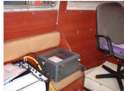
Odom Hydrotrac Echosounder onboard survey boat.
