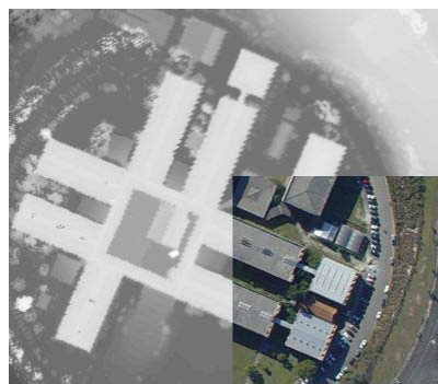
Figure 6. A part of a LIDAR intensity image is overlaid by a patch from the SONY-F717 ortho-photo.
