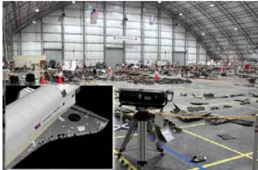
Figure 2: Trimble S10 scanner in the hangar for rebuilding the American space shuttle Columbia” and reconstruction from point clouds.
