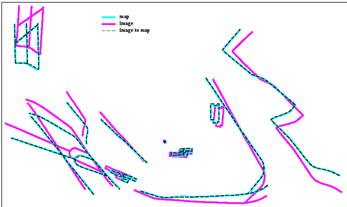
Figure 7. Registration using linear features: pre-aligned data and results
