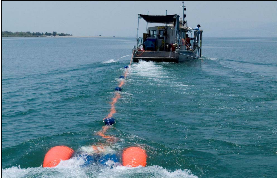
A sparker survey was carried out on a tight grid, along with multibeam with a rented ELAC SeaBeam 1180 system, and Geometrics Cesium magnetometer.
