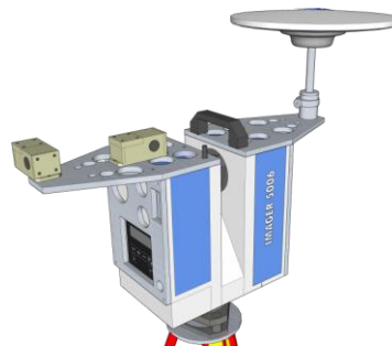
Figure 1: Actual setup of the MSS equipped with one GNSS antenna and two external inclinometers on top of a phase-based TLS
