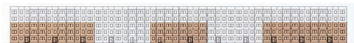
Figure 8: Partial demolition in the Dürer Quarter (in red colour: remaining parts of the building).
