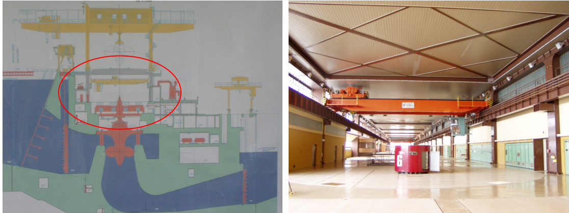
Figure 7 Cross section of the hydro-electric power plant (left) and bridge crane rail (right)
