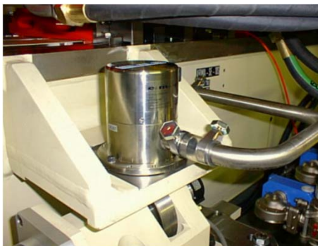
Levelsensor: Installation on girder
