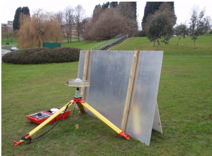
Figure 14: Antenna Set-up with Metal Reflector Sheet at pt GRASS
