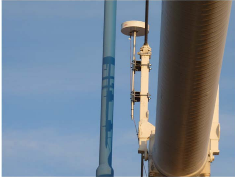
Figure 3: AT503 Antenna Attached to Main Cable on Severn Crossing Suspension Bridge
