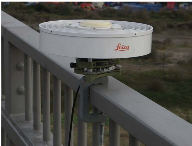
Figure 1 : GPS Antenna Set-up Showing AT503 Antenna, Clamp and Tribrach Attachment on the Avonmouth Viaduct
