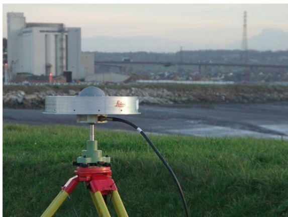
Figure 2: AT504 Choke Ring at One of the Reference Stations at the Avonmouth Harbour
