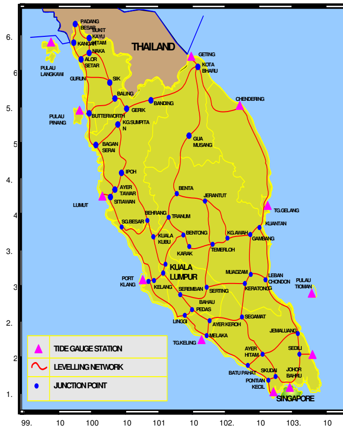
Figure 2.0 The extent of Precise Levelling Network in Peninsular Malaysia
