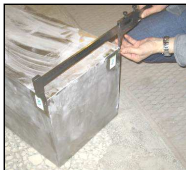
Figure 11: Survey by caliper.
