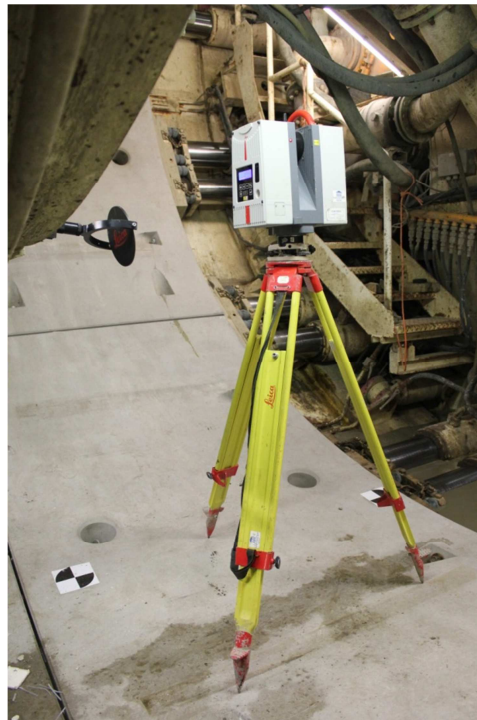
Figure 2: Terrestrial laser scanner in the TBM.
