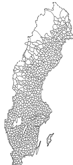
Figure 2: Levelling lines of the third precise levelling of Sweden.
