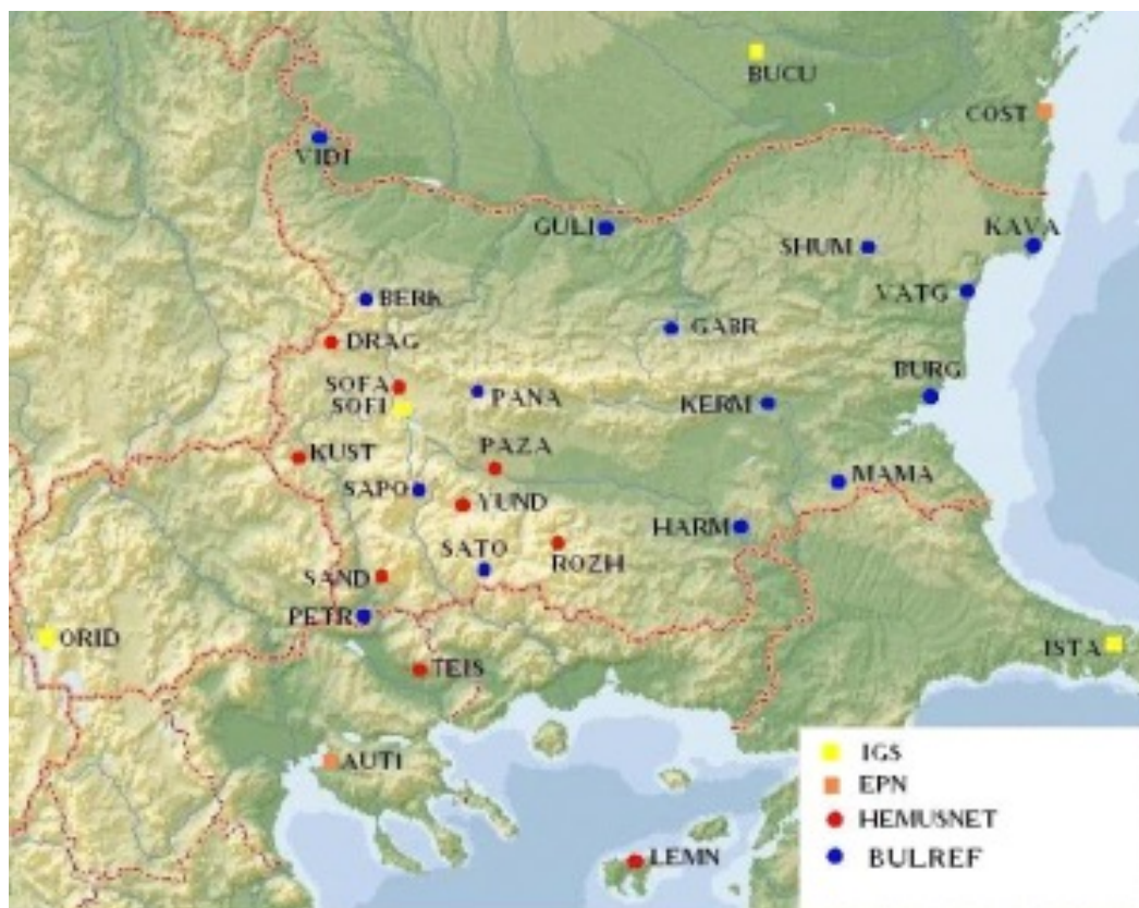
Figure 2. Locations of IGS, EPN, HemusNet and other permanent sites and BULREF point
