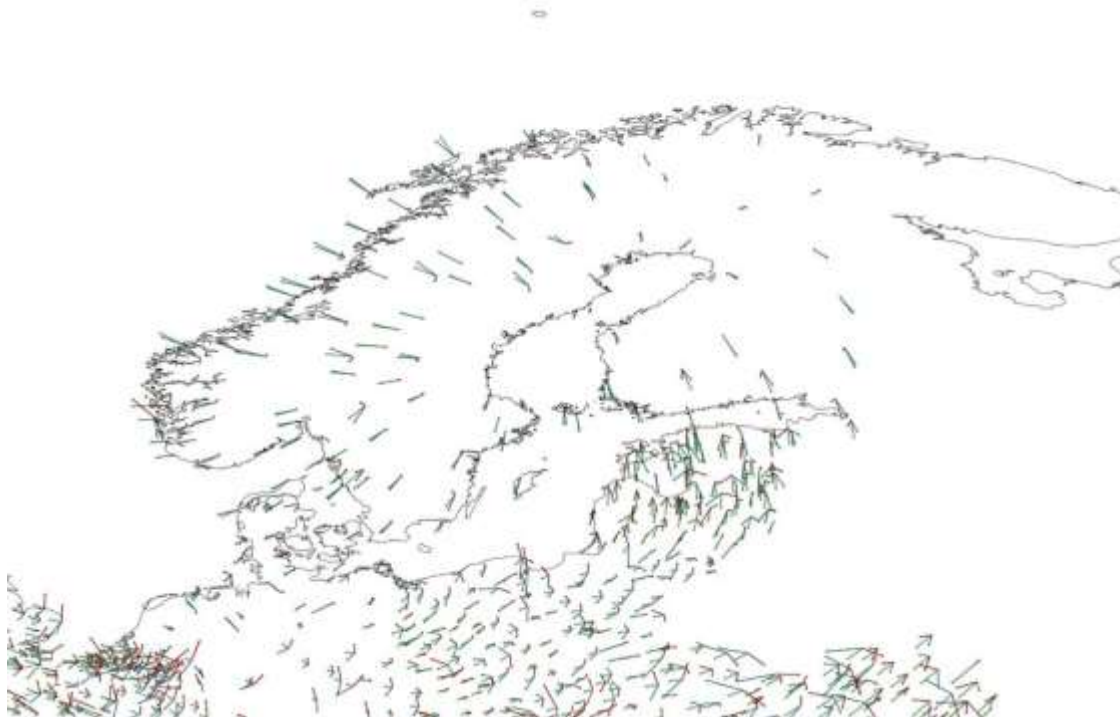
Figure 8. Model (green vectors), EPN densification (blue vectors) velocities and their difference (red vectors).
