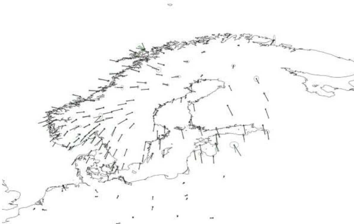
Figure 7. BIFROST (black vectors), model (green vectors) velocities and BIFROST velocity uncertainties (black ellipses).
