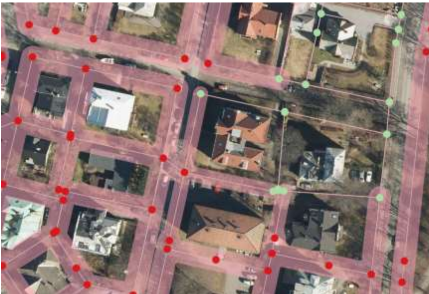
Figure 7: Situation from Oslo. Buffer showing accuracy of lines (3 times standard deviation on each side of the line), colours showing standard deviation of points (green: 8 cm, red: 100-150 cm).
