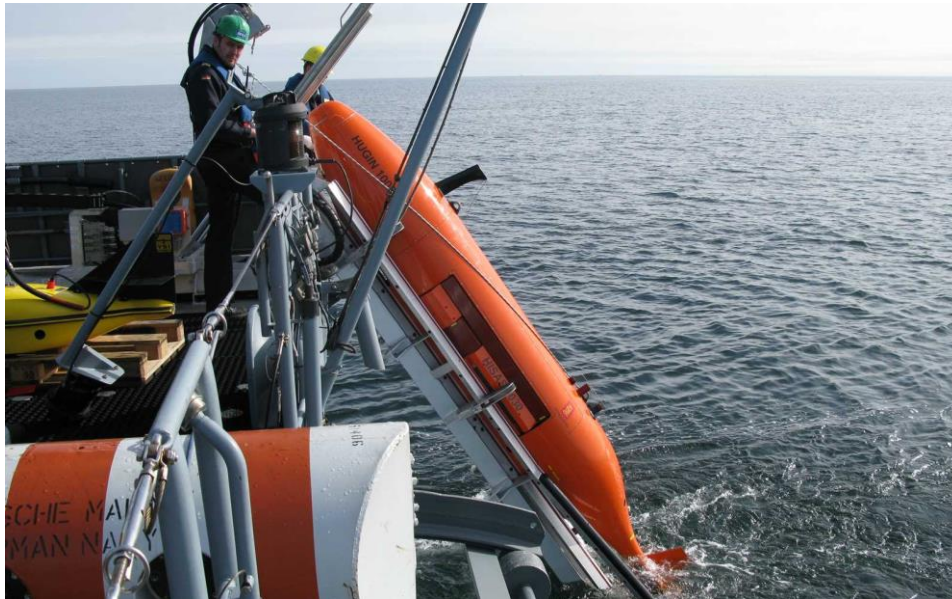
Figure 5: Autonomous Underwater Vehicle HUGIN produced by the Kongsberg Maritime. https://www.kongsberg.com/maritime/products/marine-robotics/autonomous-underwater-vehicles/AUV-hugin-superior/
