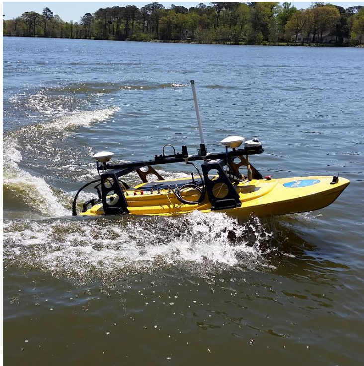
Figure 4: Unmanned surface vessel Teledyne Oceanscience Z-Boat 1800RP http://www.teledynemarine.com/z-boat-1800rp
