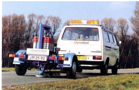
Falling Weight Deflectometer (FWD)
