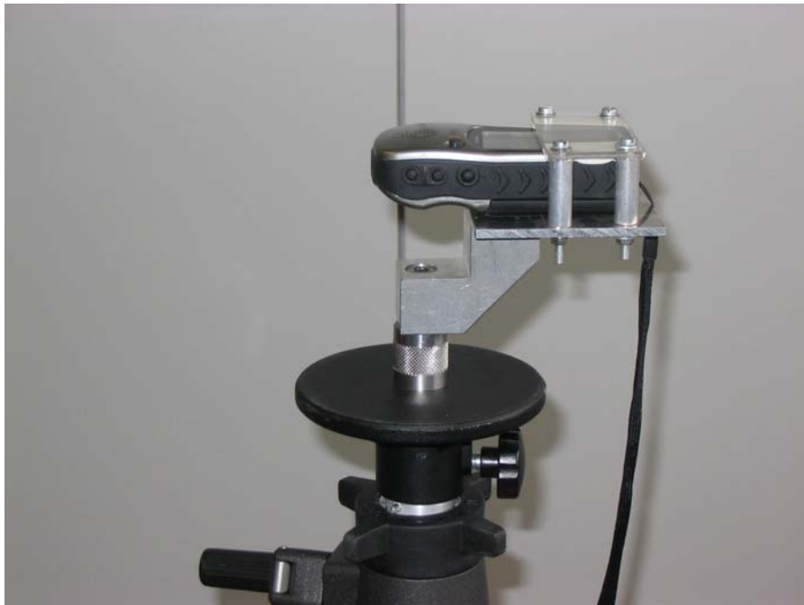
Figure 2: Garmin eTrex Vista and adapter for tribrack
