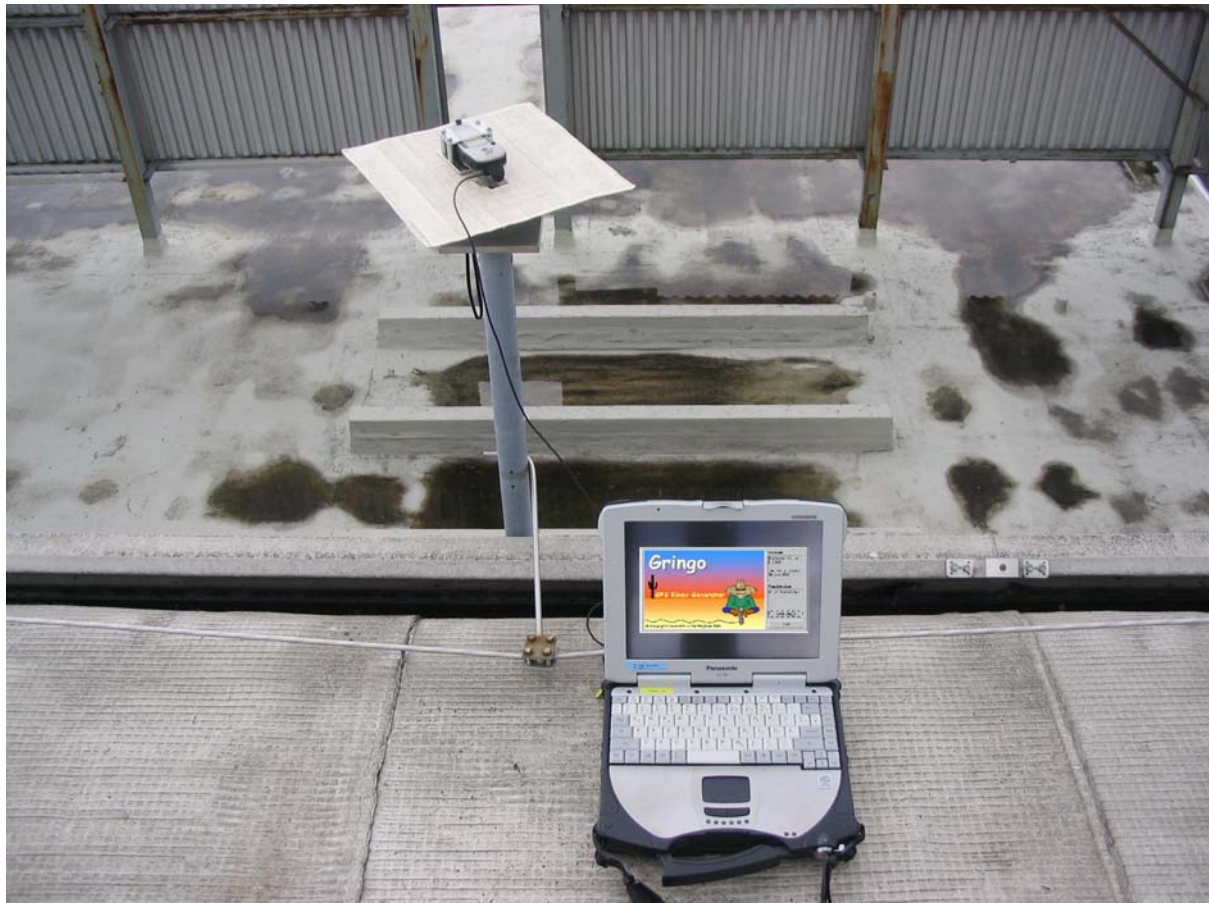
Figure 1: GARMIN eTrex Vista, laptop and shielding against multipath effects
