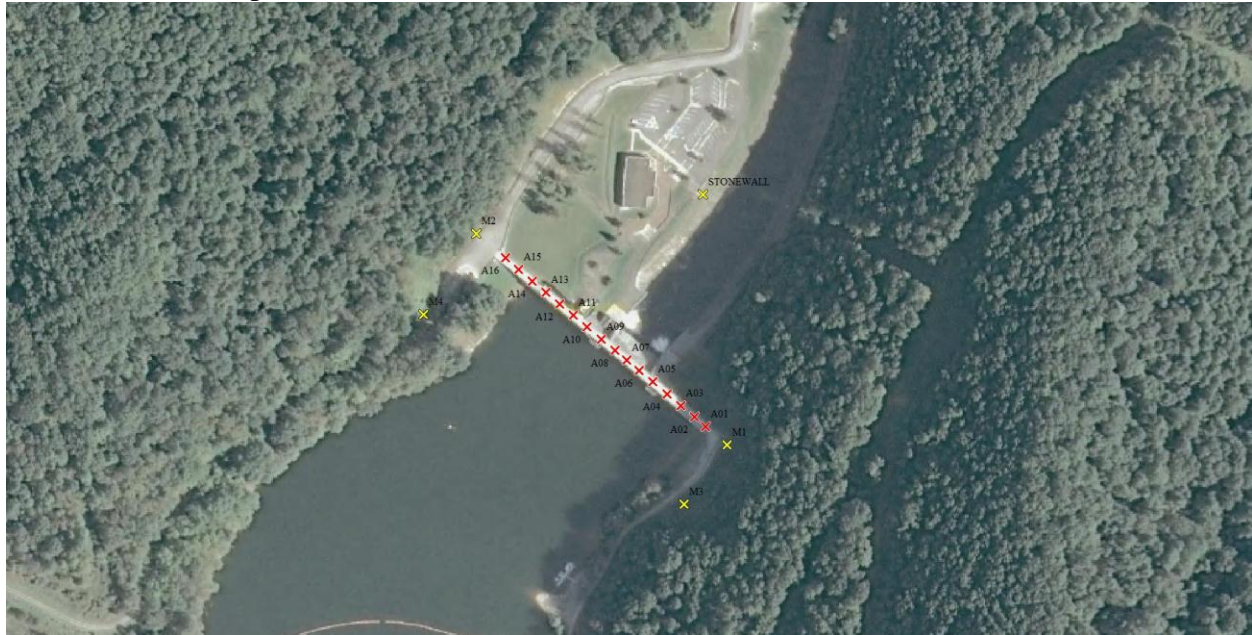
Figure 8 -Concrete Gravity Dam network
