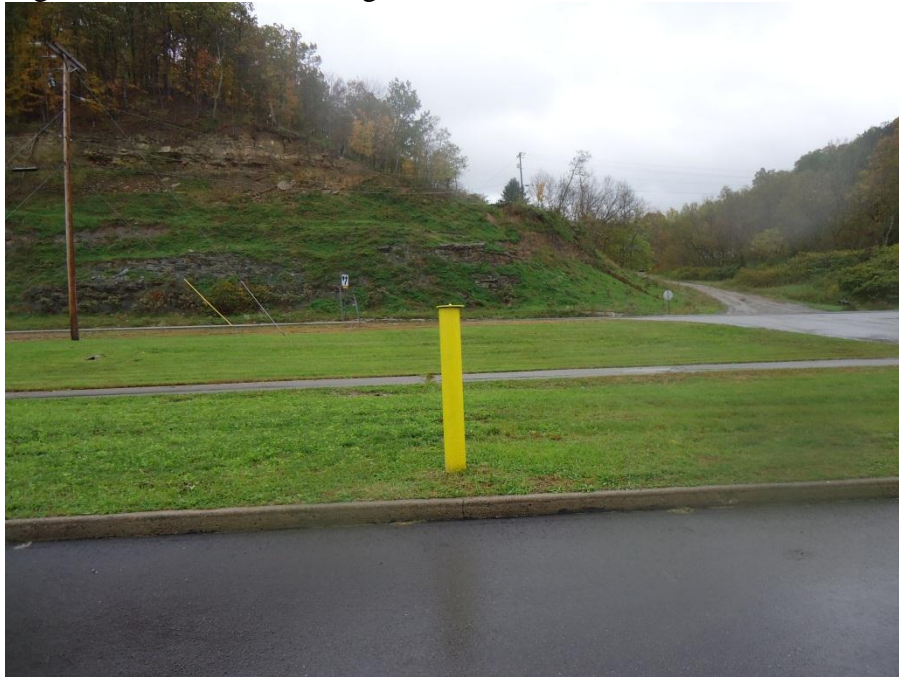
Figure 3 - Reference Monument pedestal
