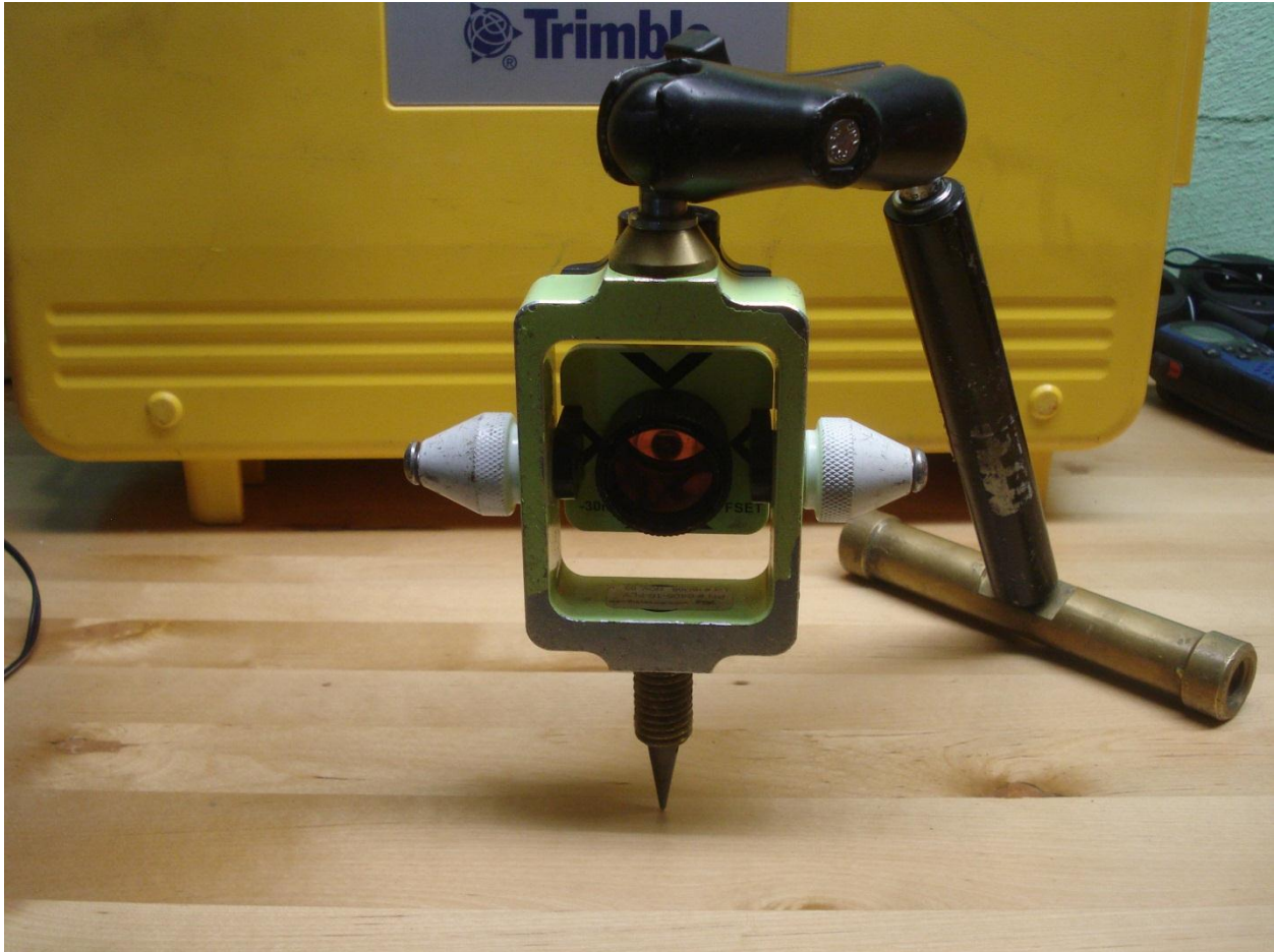
Figure 13 - mini prism with monopole
