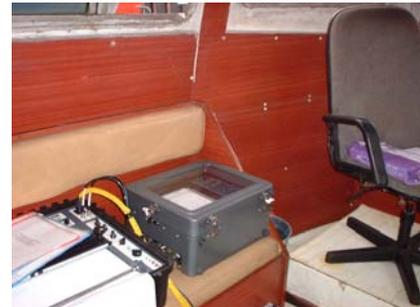
*Odom Hydrotrac Echosounder onboard survey boat.*
