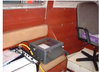
*Odom Hydrotrac Echosounder onboard survey boat.*
