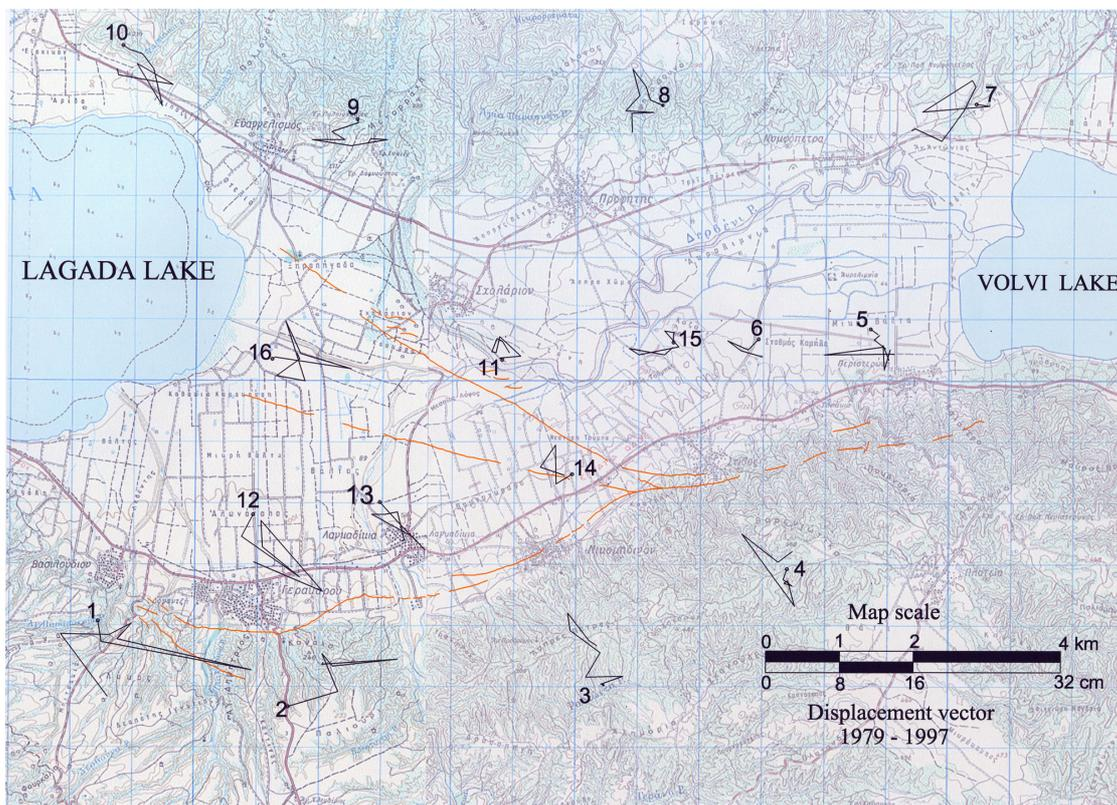
Fig. 1 The vectors of coordinate differences from 1979 until 1997 in the Volvi network
