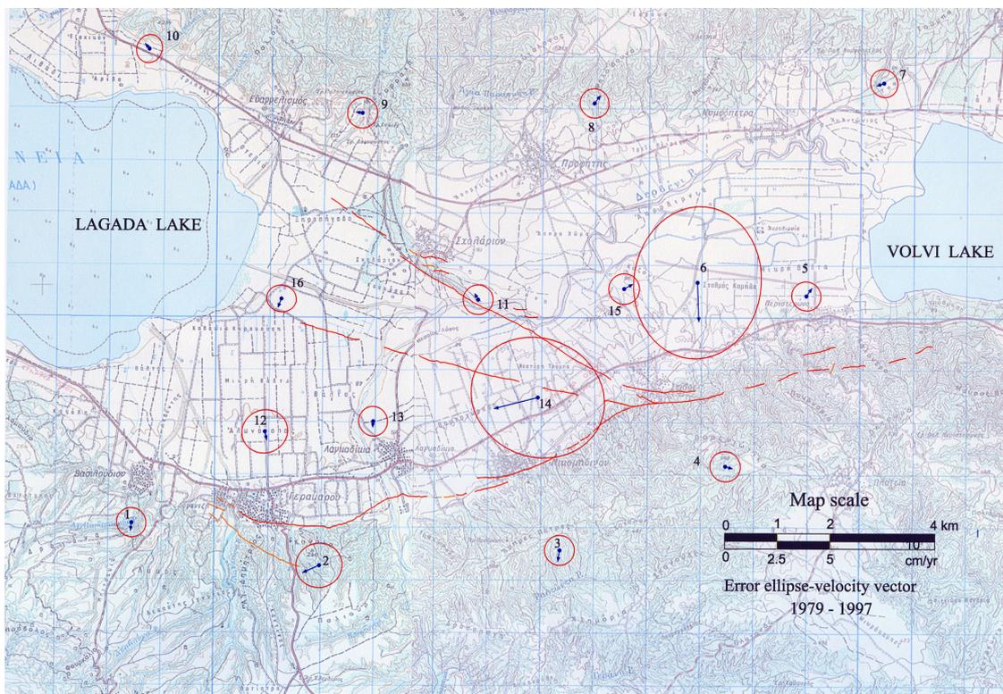
Fig 4. Velocity vectors and their confidence error ellipses ( $1-\alpha=0.95$ ), for the Volvi Network as results from the measurements in the years 1979, 1981, 1982, 1983, 1989, 1990 (classical network) and 1995, 1997 (GPS Network).
