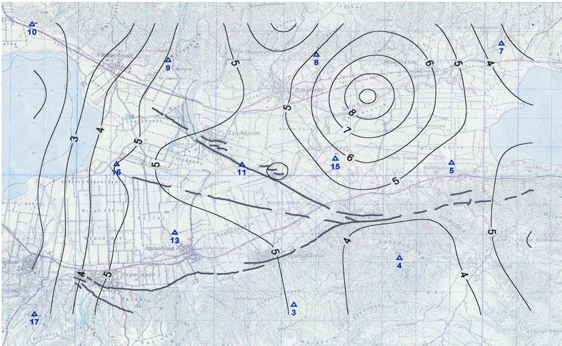
Fig. 3. The maximum shear strain  $\gamma$  ( $\gamma \times 10^{-6}$ ) between epochs 1995 –1997 of Volvi network using the collocation method with mean distance  $R=4$  km.
