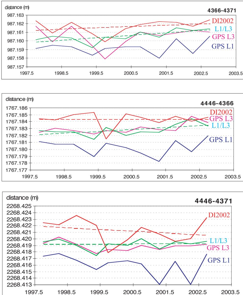
Fig. 3. Comparison GPS and EDM derived distances
