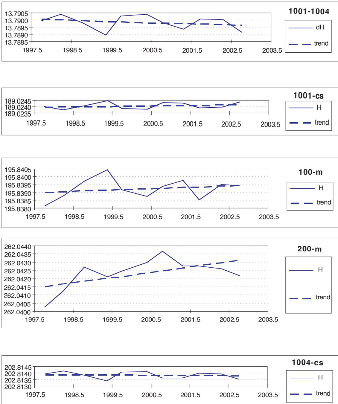
Fig. 2. Graphic interpretation of the measured relative height changes
