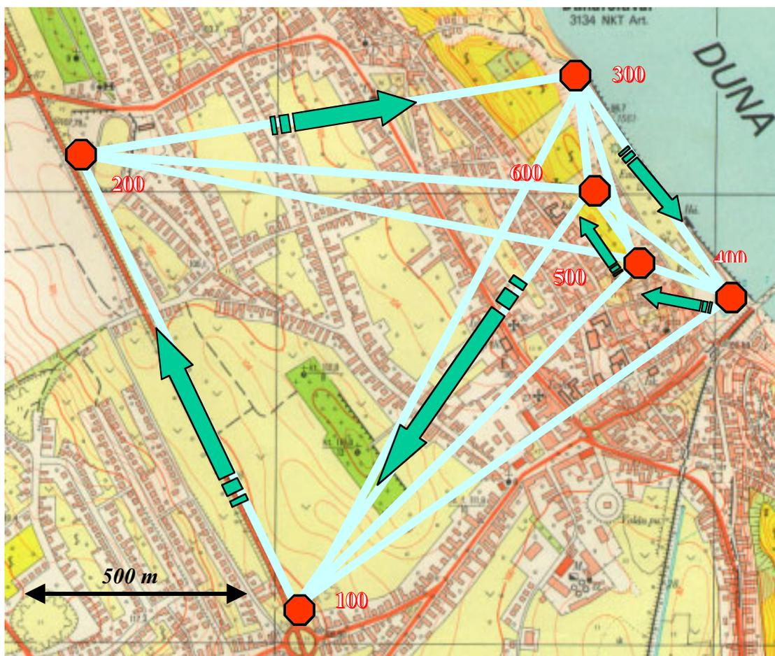
Fig. 4. The full roving GPS observation scheme
