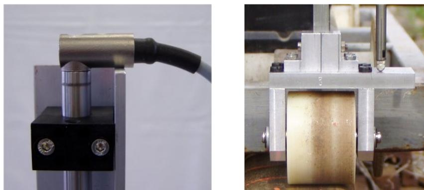
Figure 4. The WA100 sensor protection
