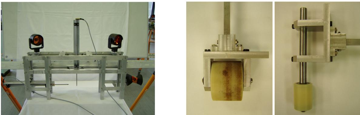
Figure 3. The bearing structure of the system (left) and mechanism of vertical guide wheels (middle) and horizontal guide wheels (right)
