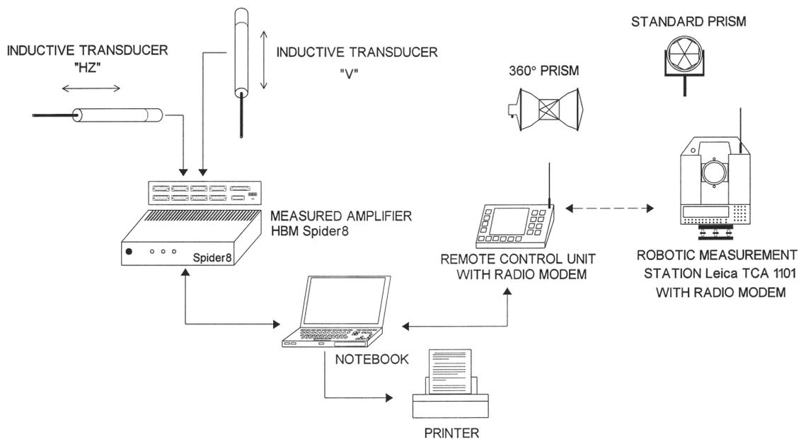
Figure 1. Connection scheme of the measurement system
