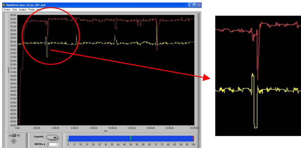
Figure 9. Changes in distances measured by sensor after transition of the rail dilatation
