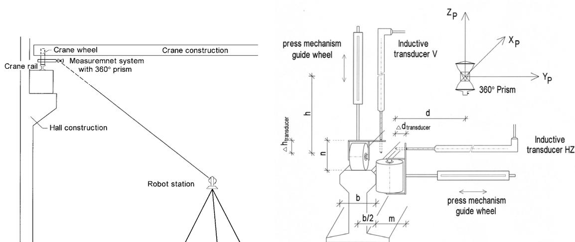
Figure 6. Determination of 3D position of the observed point
