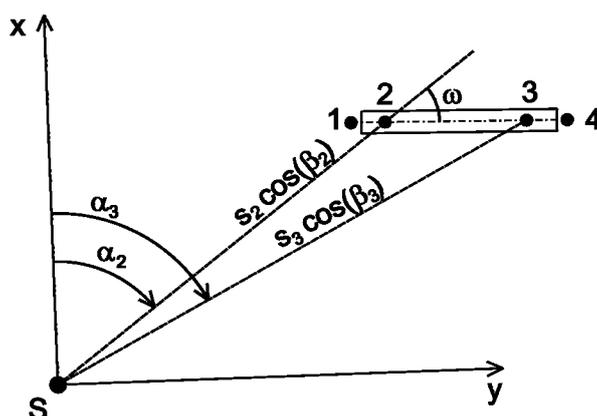
Figure 7. Determination of the 3D position of observed point
