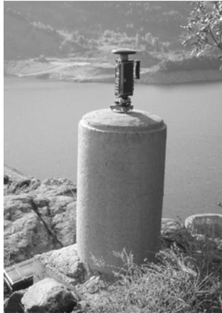
Figure 2: Reference point with Thales Z-MAX GPS
