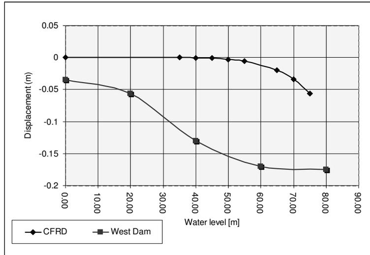
Figure 4: Vertical displacement of crest during filling up a reservoir
