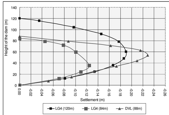
Figure 3: The calculated settlements at the end of construction of DVL and LGC dams
