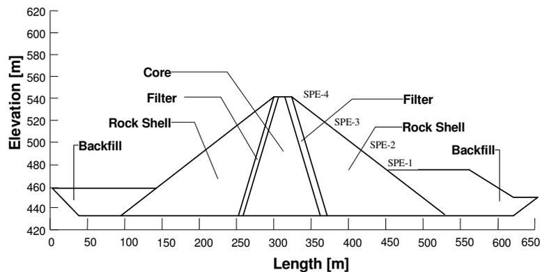
Figure 1. Schematic cross-section of the West Dam
