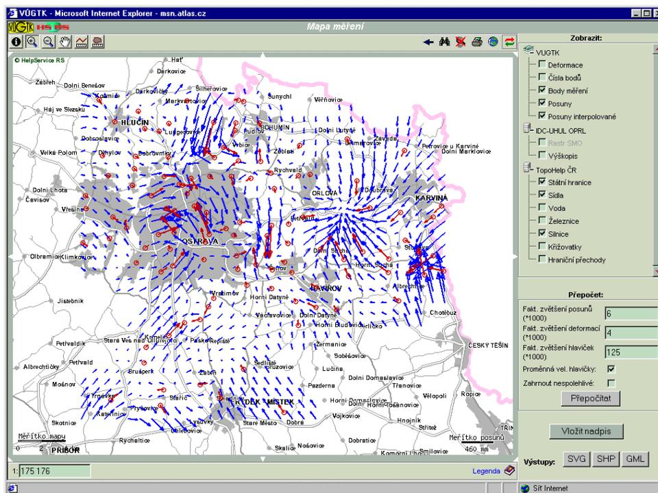
Figure 2: Resulting interpolated movements of Ostrava network
