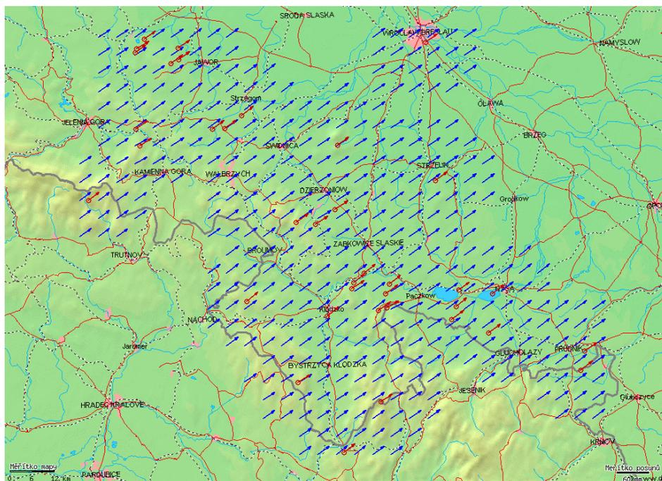
Figure 4: Measured displacements in ITRF
