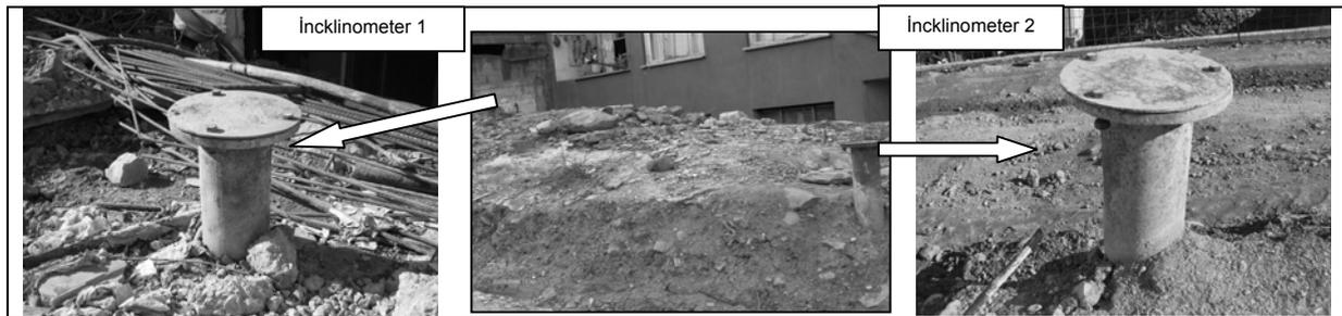
Figure 6: Inclinometer pipe and instrument installed on tunnel
