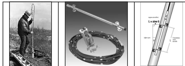
Figure 5: Settlement and Measurement of Inclinometer
