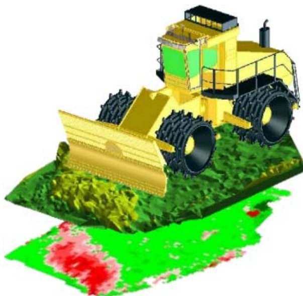
Figure 2: Compactor on a landfill with sensor head
