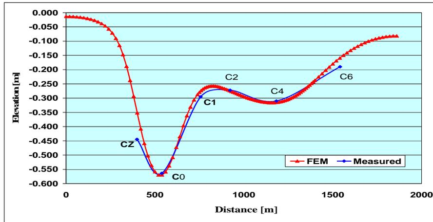
Fig.6: Measured and FEM Surface Subsidence
