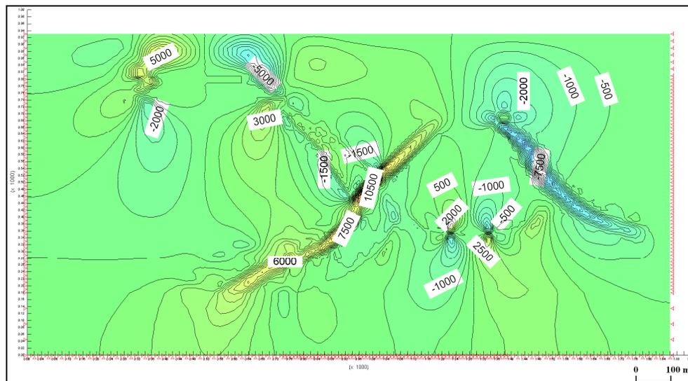
Fig. 7 - Distribution of maximum shearing stress (MPa)
