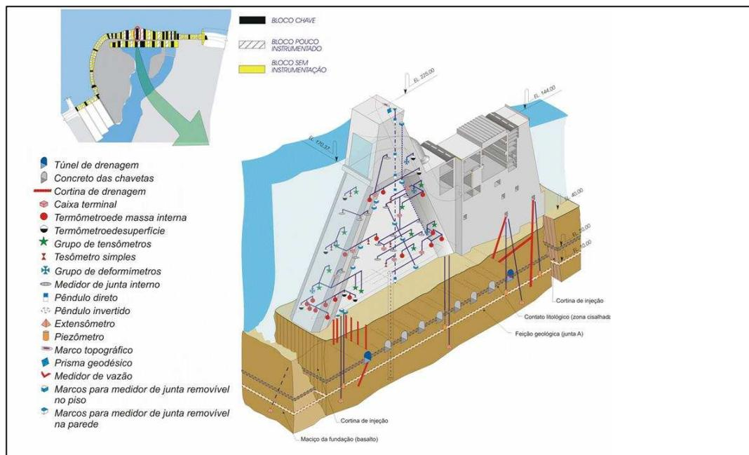
Figure 5 - Instrumented key block at ITAIPU dam
