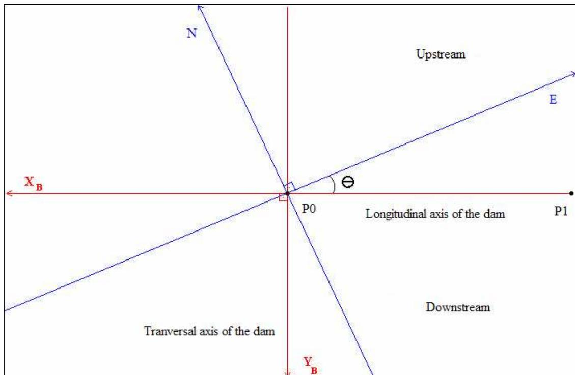
Figure 8 - Situation between the UTM system and the Dam Axis system.
