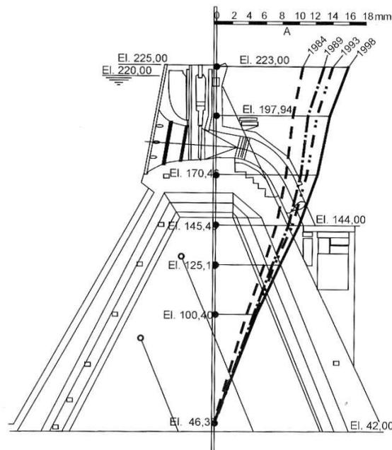
Figure 6 - Observations conducted by the Plumb line installed at the F19 point.
