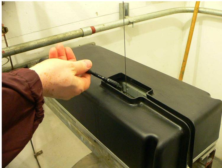
Figure 4 - Automated reading (ADAS) of the plumb line at ITAIPU dam
