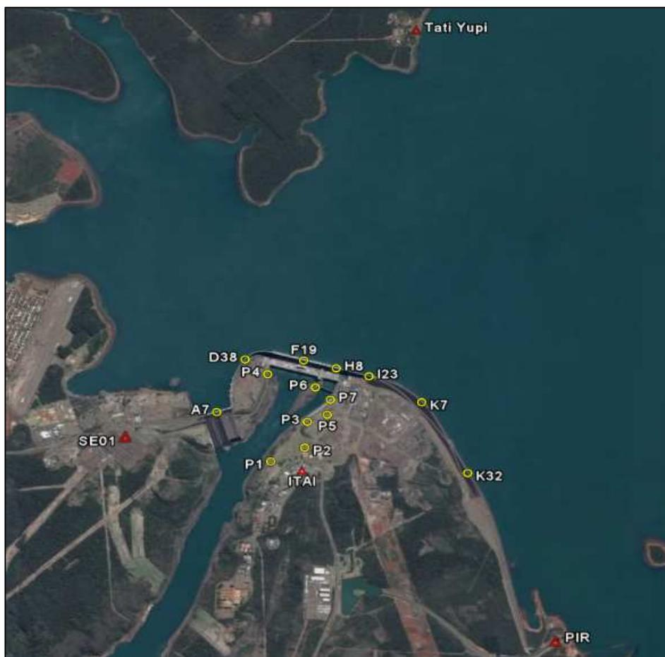
Figure 7 - Network of pillars and points on the dam, particularly, F19
