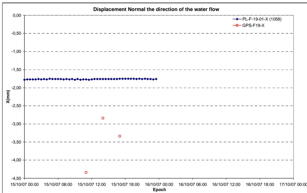
Graph 4 - Displacements in the normal direction of the water flow (X) of point F19 determined by GPS (2<sup>nd</sup> campaign) and by direct PL
