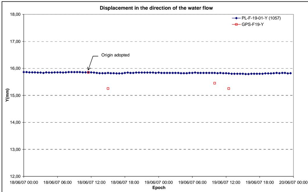
Graph 1 - Displacements in the water flow direction (Y) of point F19 determined by GPS (1<sup>st</sup> campaign) and by direct PL
