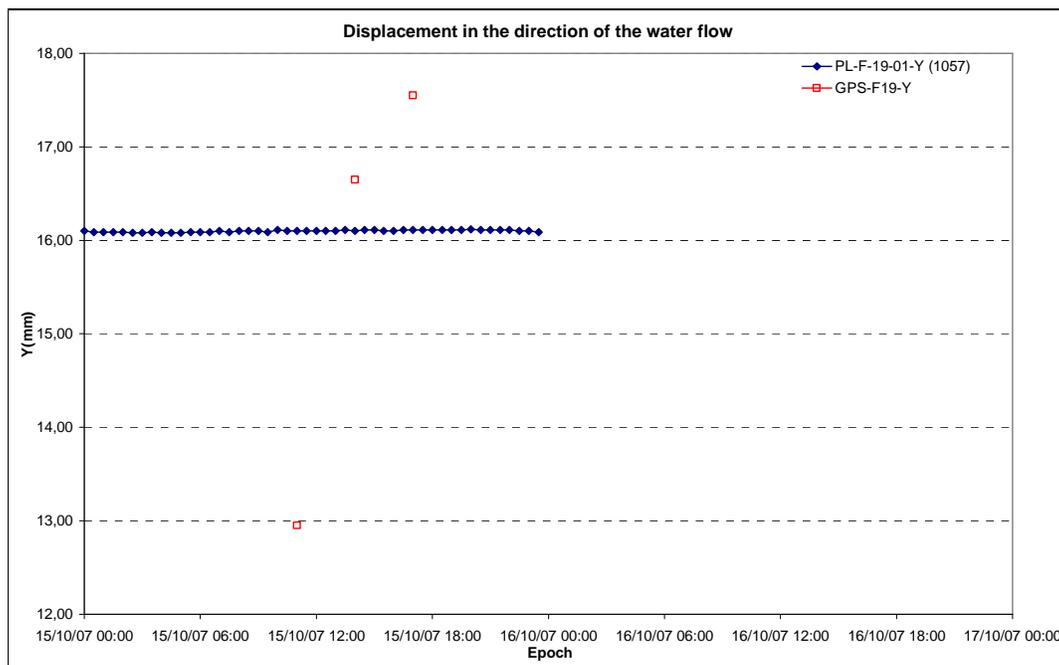
Graph 3 - Displacements in the direction of the water flow (Y) of point F19 determined by GPS (2<sup>nd</sup> campaign) and with direct PL
