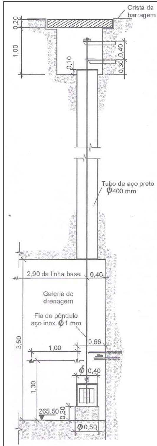
Figure 2 - Installation scheme of a plumb line in a concrete dam.
