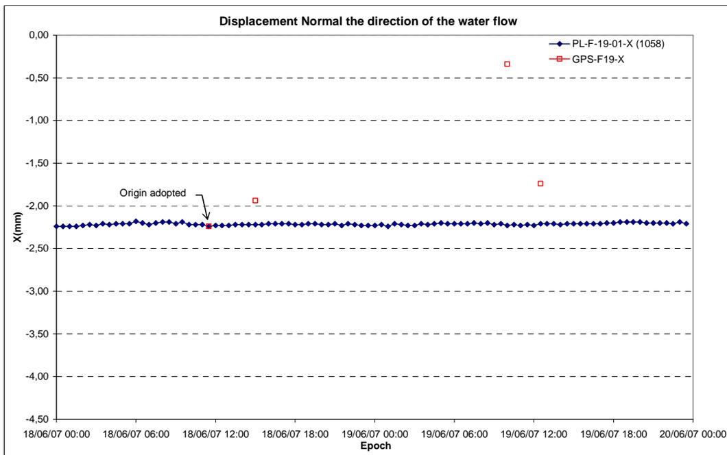
Graph 2 - Displacements in the normal direction of the water flow (X) of point F19 determined by GPS (1<sup>st</sup> campaign) and by PL
