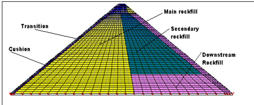
Figure 2 - Shibuya Dam, FEM mesh and dam zoning.
