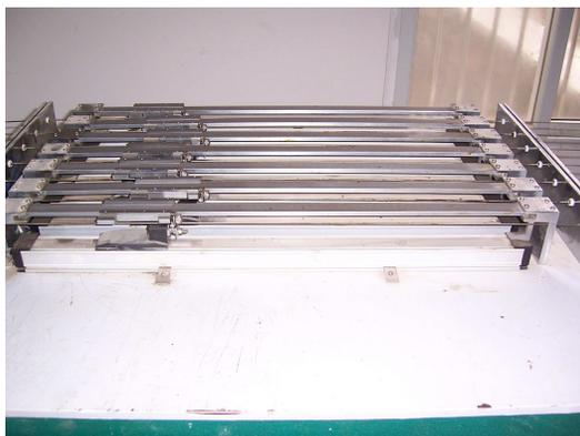
Figure 3 - Interior wire extensometer.
