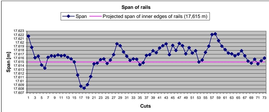
Figure 5 - Span of the crane rails
