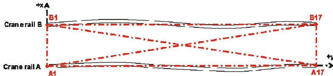
Figure 2 - Referential system of the crane rail
