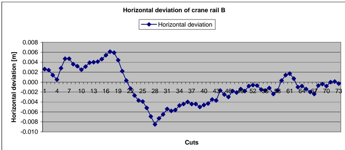
Figure 6 - Horizontal deviations of the crane rail B
