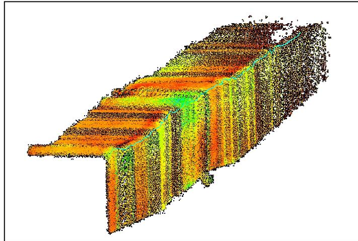
Figure 4 - Point cloud of the left rail with length 80 m with the modelled inner edge
