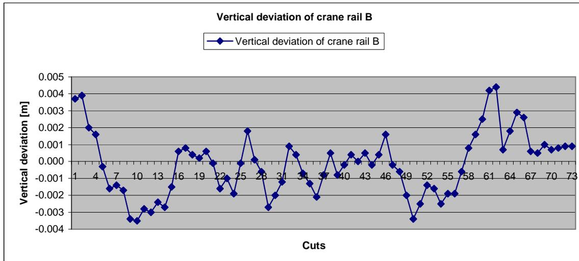
Figure 7 - Vertical deviation of the crane rail B
