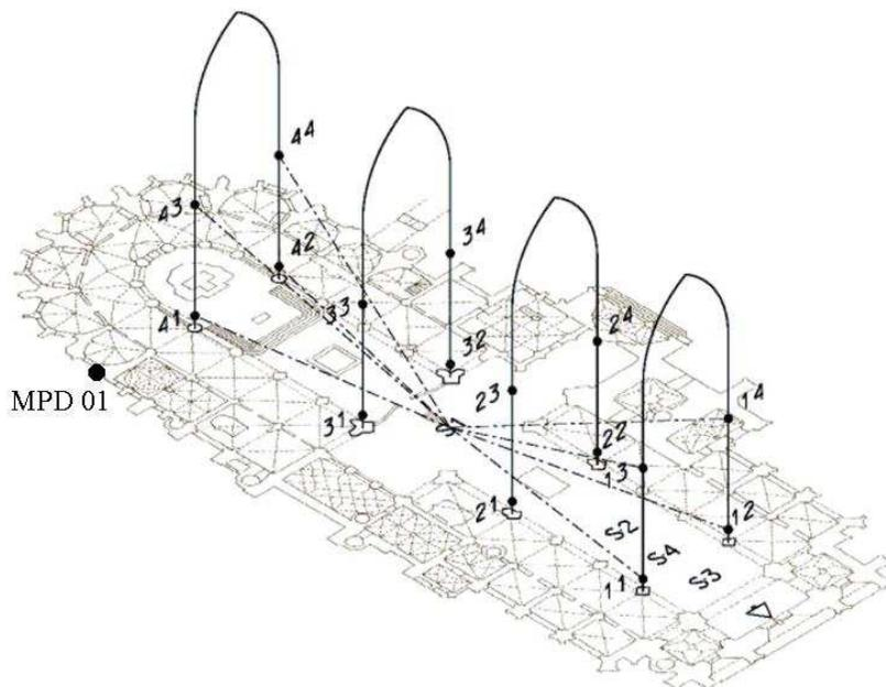
Figure 2 - Deployment of measuring points in the St. Vitus Cathedral
