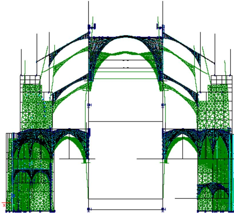
Figure 5 - Displacements of the section of the St. Vitus Cathedral – numerical model in Feat
