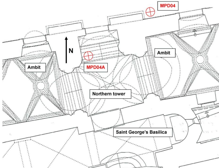
Figure 6 - Site plan with instrumented boreholes in northern tower of the St. George's Basilica
