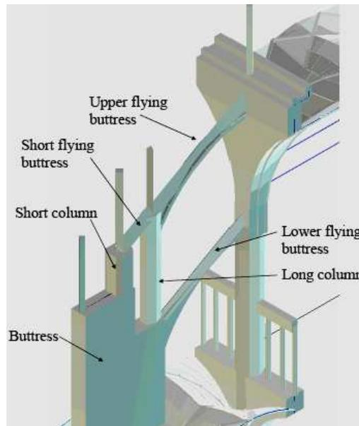
Figure 3 - Detail of bearing system of the St. Vitus Cathedral
