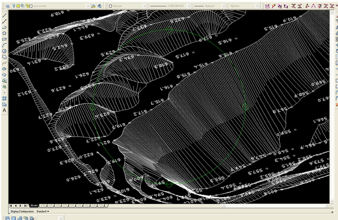
Figure 4: A topographic plan of opencast colliery compiled by scan data
