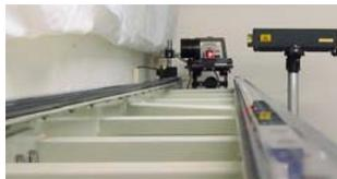
Laser interference comparator
