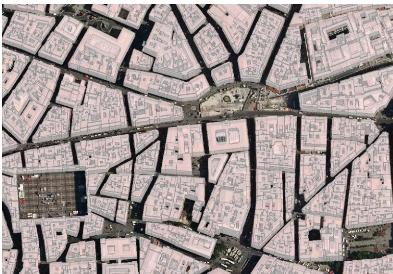
Figure 8. Superposition of the WMS service of cadastre with the orthophoto
