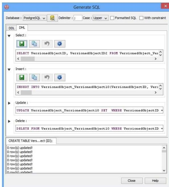
**Figure 13. Interface to select, insert, update and delete information in the database**
