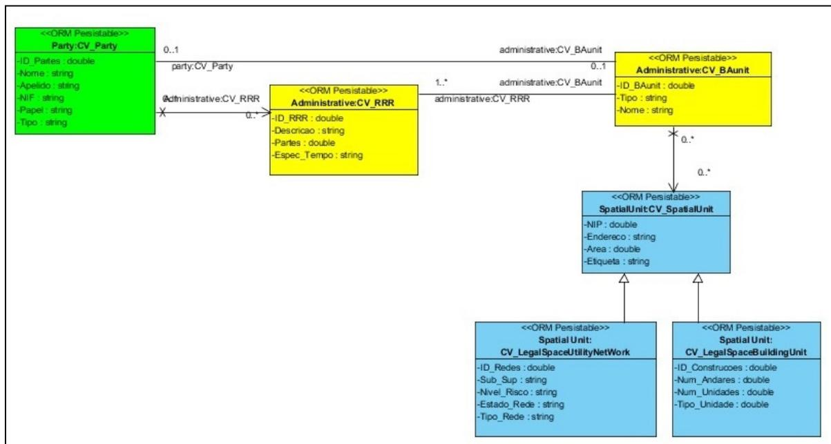
**Figure 3. Basic Classes of the CV\_Spatial Unit Package and their relationships**
