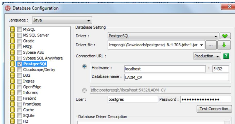
Figure 9. Configuration of the Visual Paradigm connection with the Postgres
