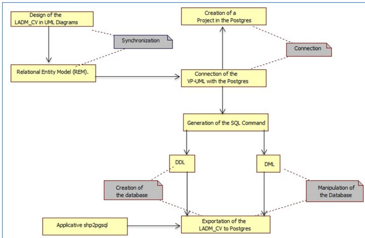
Figure 5. Flowchart showing the specification of the LADM\_CV in a relational database
