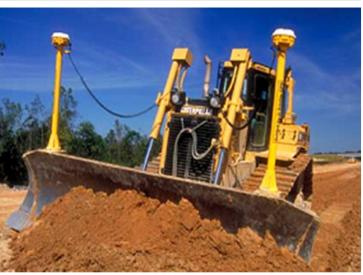
Automation becomes pervasive in most applications, supported by reliable and accurate (GNSS) positioning information, however...
