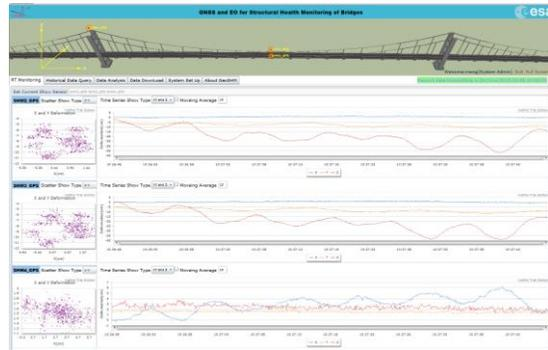
**Fig. 6** An interface that shows real-time 3D deformations
