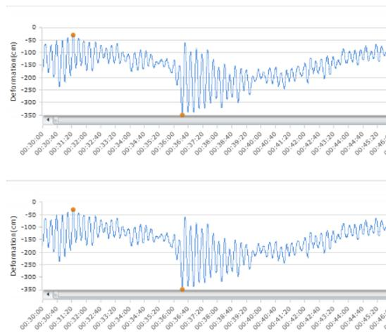
**Fig.7** Lateral deformations measured by SHM2 and SHM3 under wind loading of 41m/s
