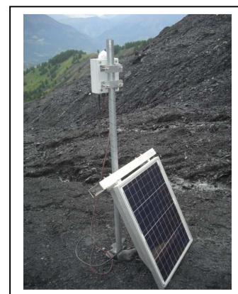
Fig. 6 Geomon low-cost GNSS receiver and its solar panel on the Super-Sauze landslide (Boetzlé, 2015).
