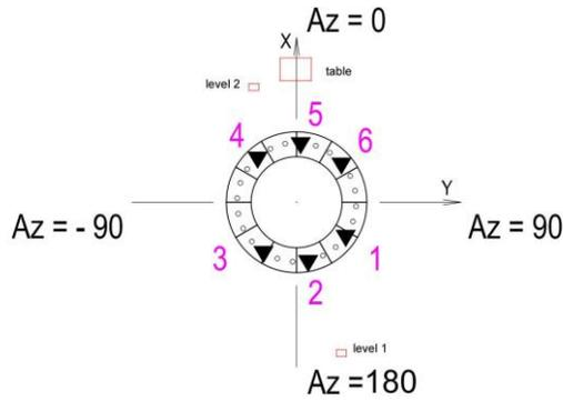
**Fig. 3** Diagram of the distribution of the foundation controlled points.
