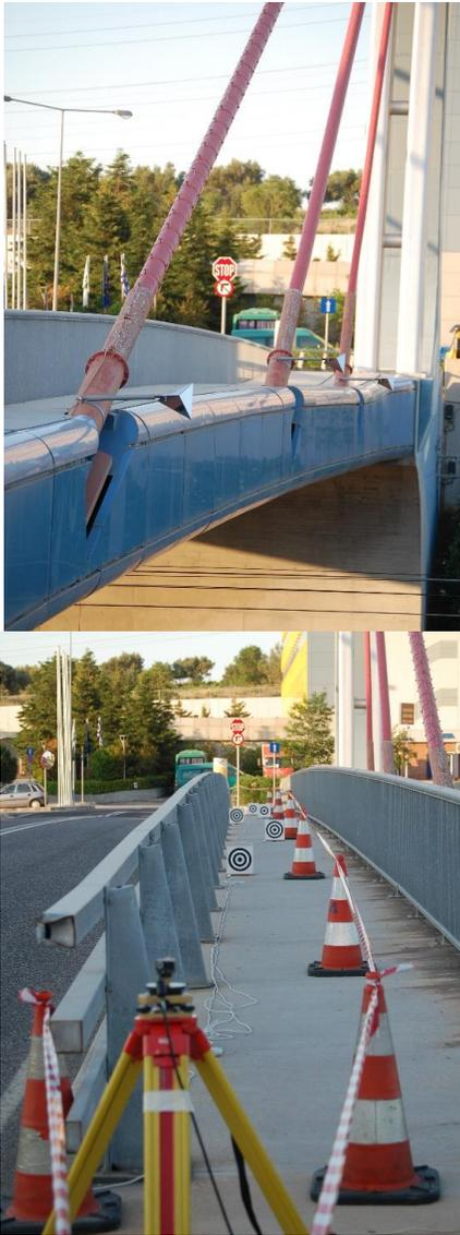
**Fig. 2** GBMI corner targets fixed by the cable anchor points (up), and DIC ring-type targets placed along each sidewalk of the bridge (down).
