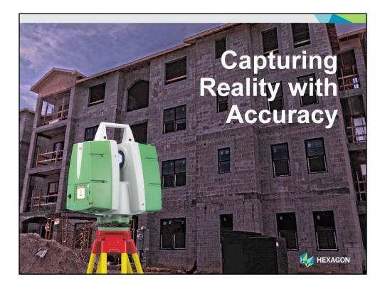
Once a project moves to the design phase, contractors are increasingly looking for ways to increase the accuracy of their models and visually convey information with the project stakeholders. The use of laser scanning to capture reality and communicate accurate as-built information is growing, bolstered by advances in hardware and software that make it faster and easier to create highvalue deliverables.
