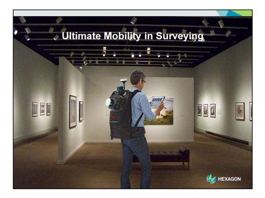
Vast strides have also been made in wearable technologies, which provide amazing flexibility and ease of use, allowing you to easily scan and map indoor or outdoor environments by simply taking a walk. Positioning is provided by SLAM technology which is basically a Photogrammetric technique that uses overlapping images to compute the sensors position and register the data.
