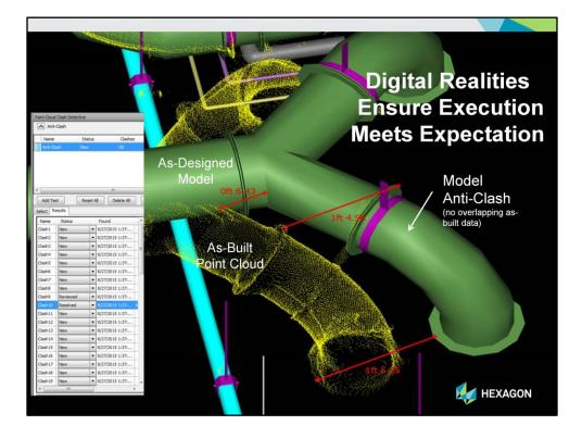
For many years the application of "clash" was a big driver for the use of scanning. Clash is where we insert the design of digital model to the existing as-built to see where the construction process may have a problem – the next big thing in construction mapping is ANTICLASH- where the post construction is compared to the digital world to be sure the construction built was to the original design. This is also referred to as Validation
