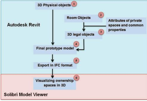
Figure 12, Development process of the prototype BIM model
