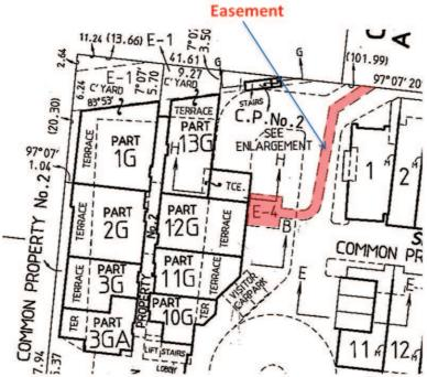
Figure 10, An easement object in a complex building development (Reeds Consulting, 2015)
