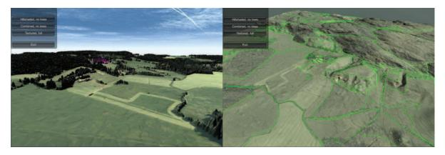
The 3D terrain model is designed using all available LIDAR data and textured with aerial photos. Hill shading and aerial photos have been combined to get a better view of the area. The green lines mark the property boundaries for the area.
